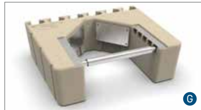
ADJUSTABLE PILING BRACKET Heavy-duty one-piece polyethylene bracket allows lateral position adjustment to attach to piles from 6"-18" in diameter. Bracket comes with two pairs of couplers with composite hardware.
