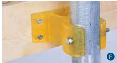
POLY PIPE STAND-OFF BRACKET Polyurethane bracket attaches top of pipe to stationary docks. Fits pipe from 2.5" to 3.5" O.D.
